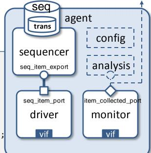
Only the connection between sequencer and driver is made here. Connection of driver and monitor to the DUT is done via the configuration mechanism
